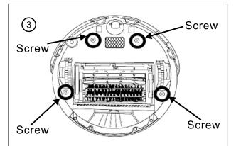
Loosen the four screws as shown in above diagram by using a Phillips head (+) screwdriver.
