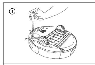
Use a Phillips head (+) screwdriver to loosen the screw that hold the side brush which is located at the top left-hand corner of the bottom casing.
