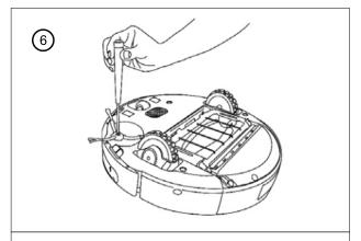
Reinstall the bottom casing and the side brush using the original screws. The device is now ready for use.
