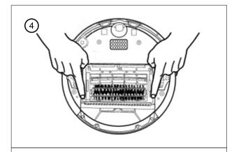
Remove the bottom casing.
