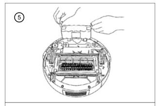
Take out the battery pack from the battery compartment and replace it with the new battery pack.
